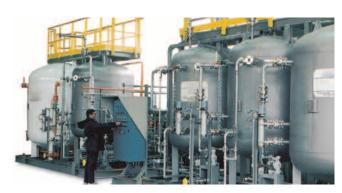
Sulphuric Acid, Biodispersant, Scale Inhibitor and Biocide Dosing Package.
